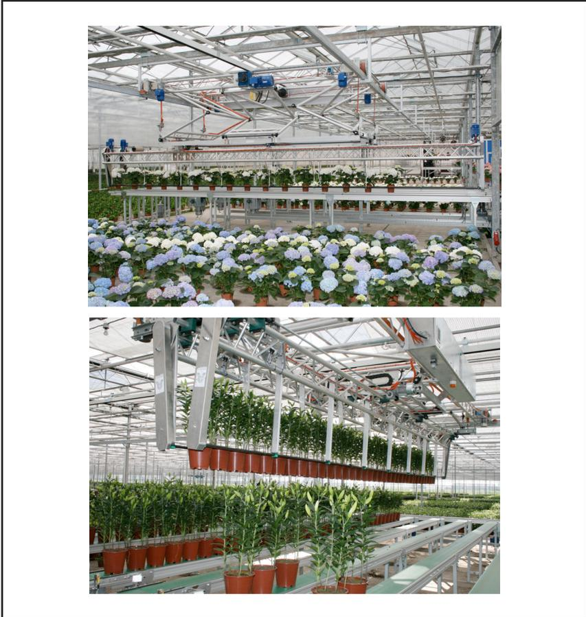
**Figures 2 and 3.** Gantry handling robots installed in pot-plant production facilities in Europe.
