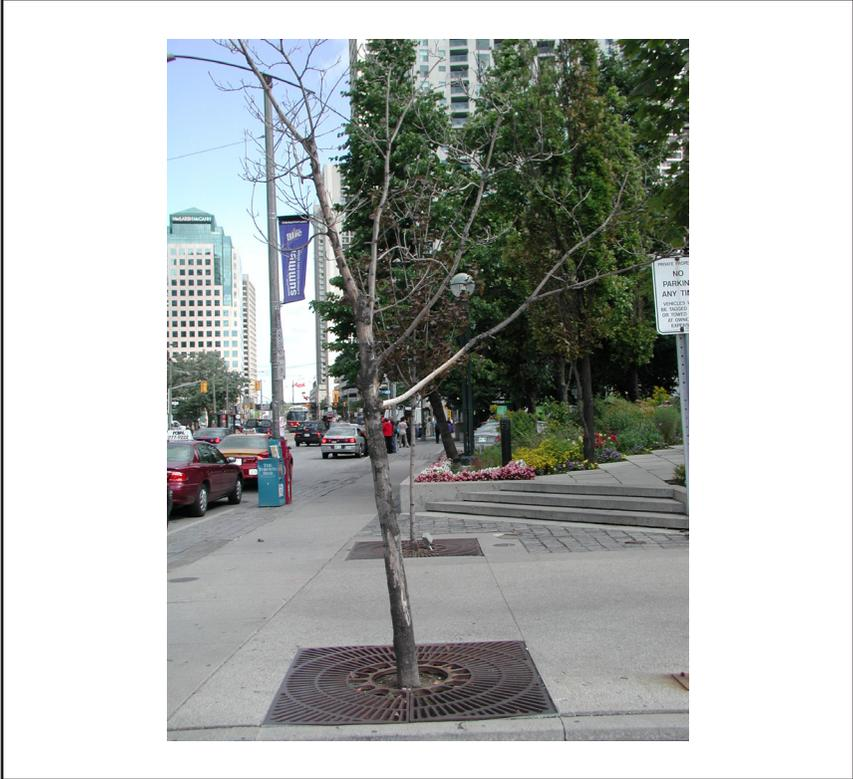
**Figure 2.** The dead tree in the foreground survived 5 years with minimal contribution to the city green space, while the group of trees in the background in a 12 × 18 m (40 × 60 ft) elevated bed had sufficient space for root growth, allowing the trees to function for a number of years.
