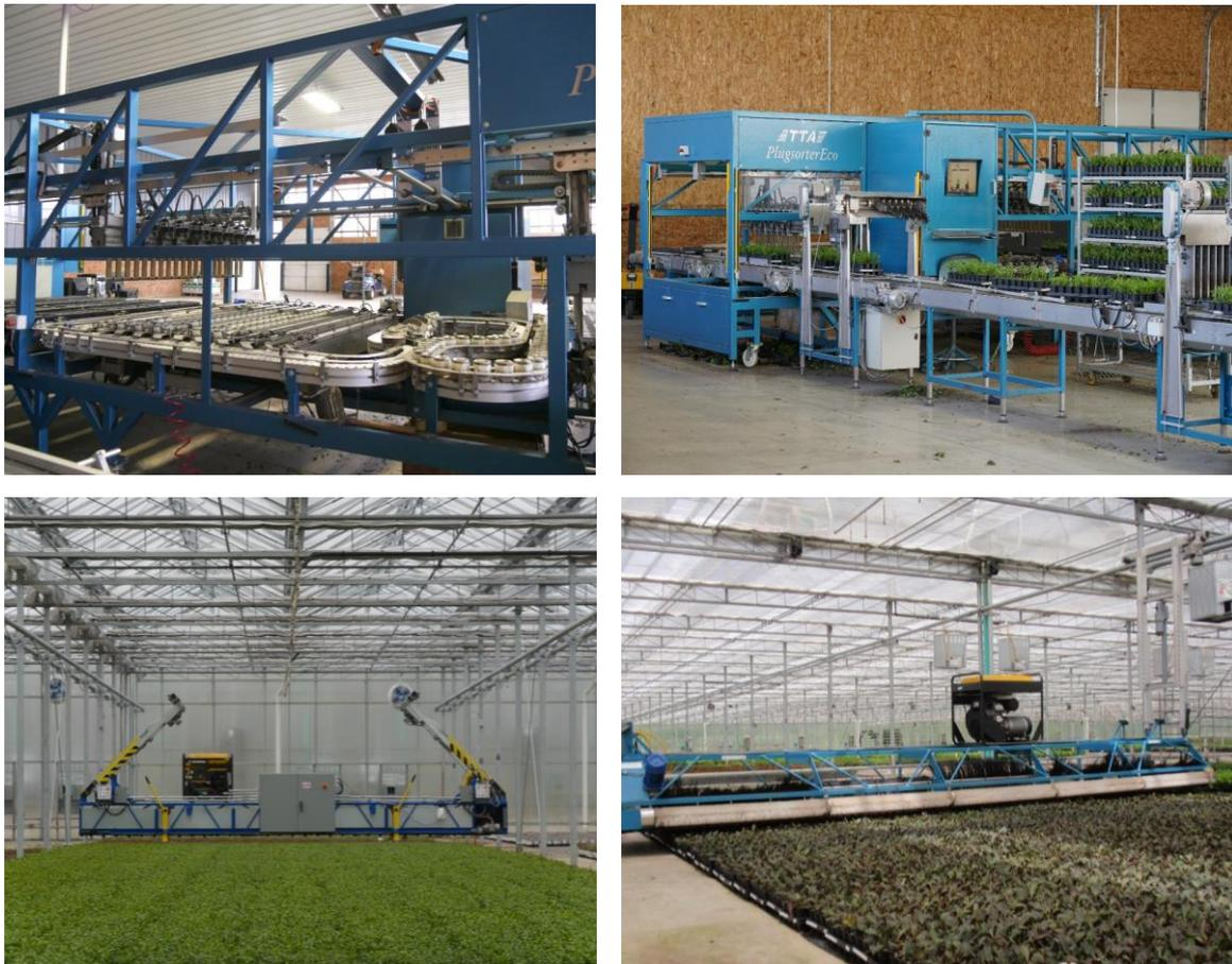
**Figure 3.** (top left, top right) sorting machine at Spring Meadow Nursery and (bottom left, bottom right) trimming machines at Spring Meadow Nursery.
