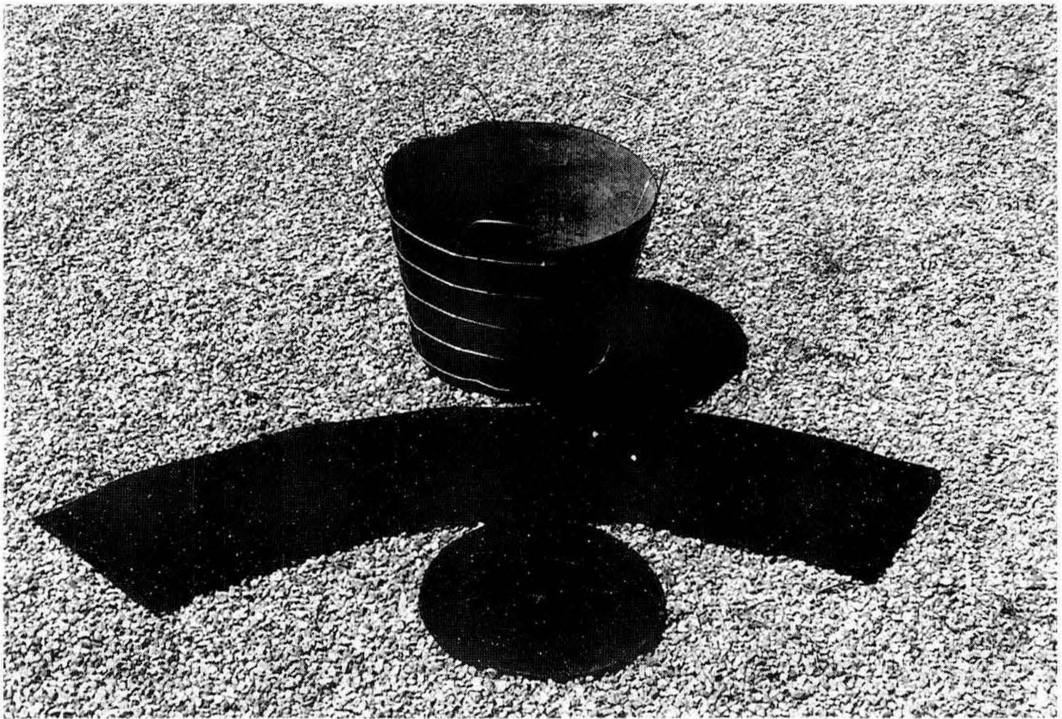
Fig. 1. The container liner, composed of two parts (circular bottom and sidewall), was designed to fit snugly inside the wire basket.
