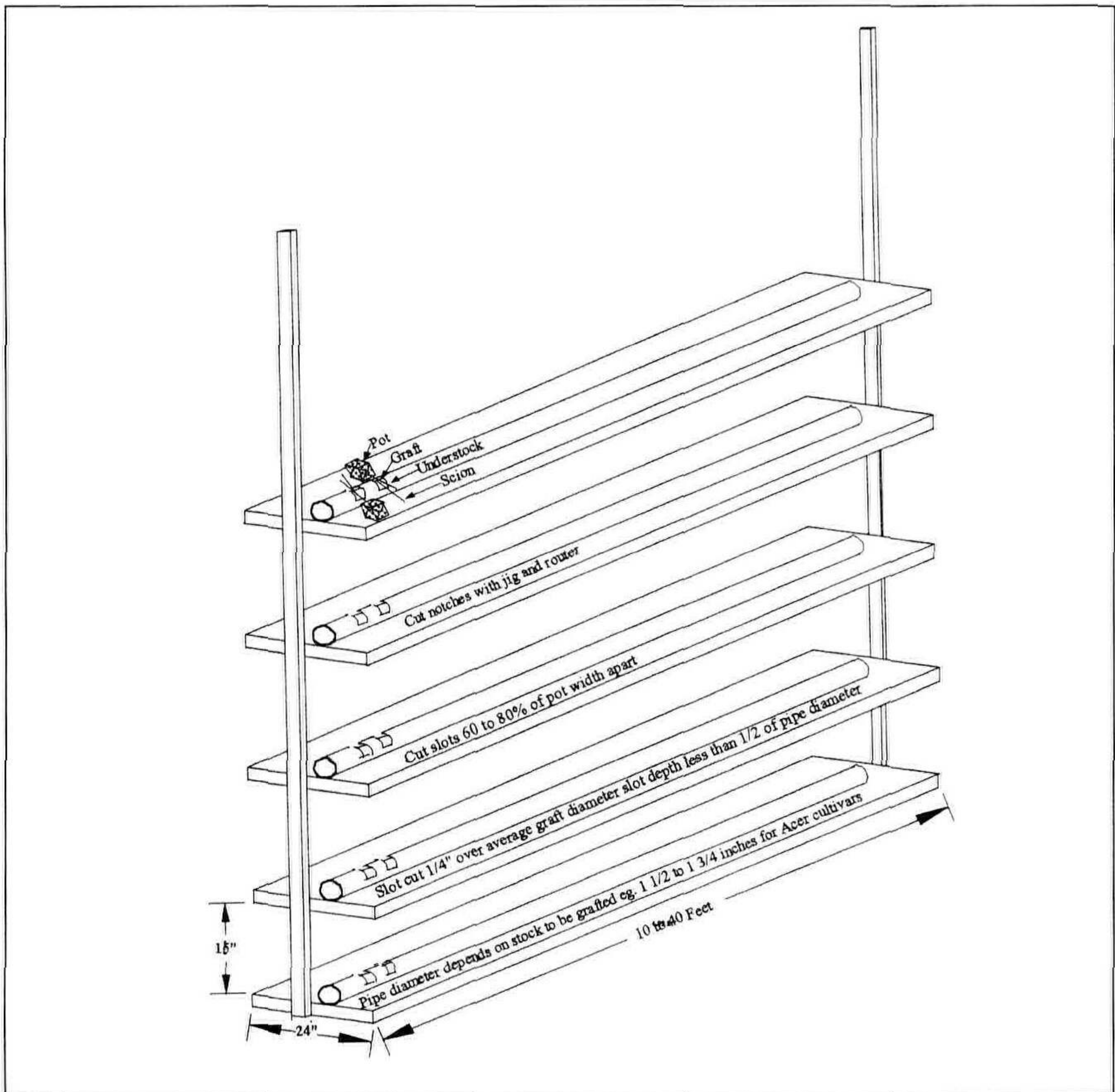
Figure 1. Pipe and shelf system developed by Mr. Frank Byles for hot-callusing the graft unions of containerized maples. The bottom shelf rests on the ground and the upright attaches to the roof. All dimensions of the system can be varied to suit the needs of the grower and/or the crop.
