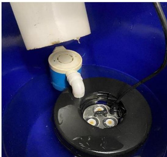
**Figure 4.** A 3-disc mist maker with float – The House of Hydro.com.
